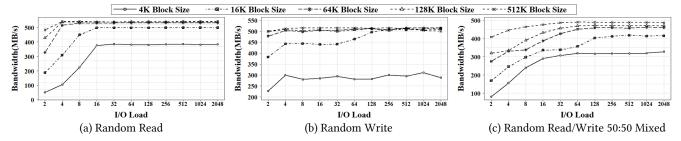
Figure 1: Performance for each block size as I/O load increases
