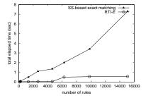
Fig. 6. Performance comparison between sequential scanning and RTI-E for exact rule matching.
